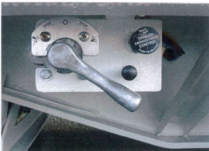
Lever shown in raise position- use for special situations only i.e. where Some extra ground clearance may be required. This height can be held by positioning the control handle at the detent half way between this position and the vertical travel position.
